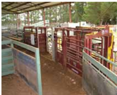
Pneumatic drafting gates in front of the crush.
